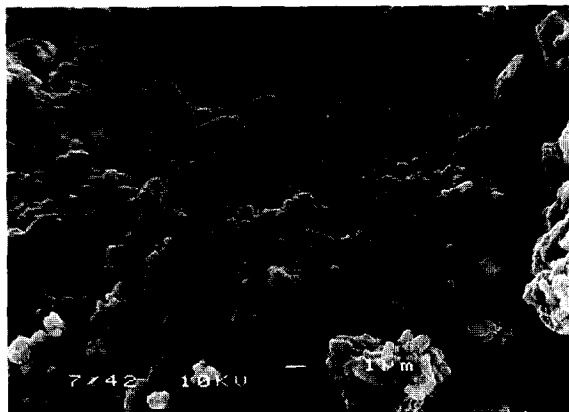
Fig. 9. Alite ( C_3S ) "rich" OPC displaying "gel" dominated microstructure.
